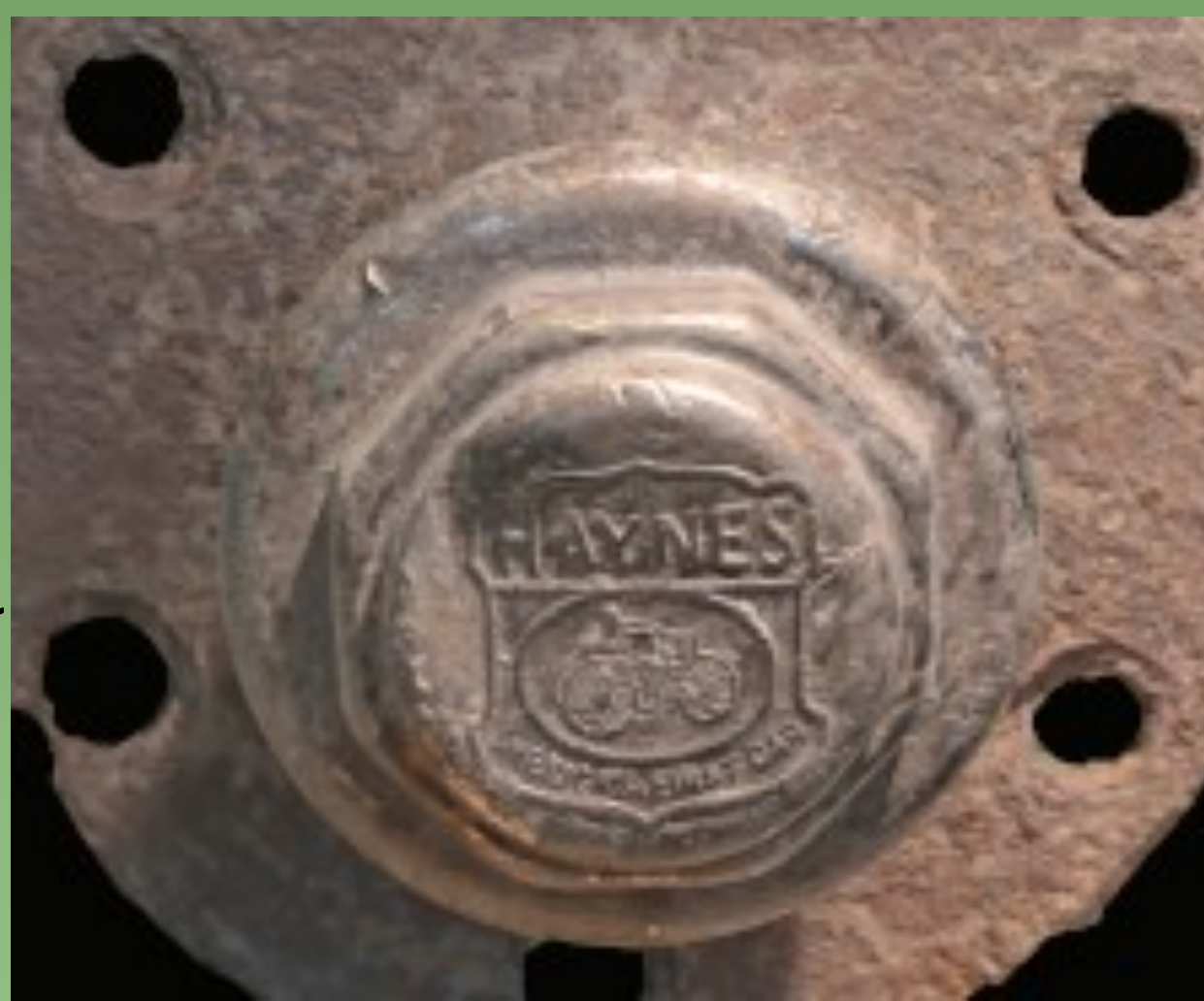
Figure 2: White metal alloy cap on the axle, with the Haynes Automobile Company logo, during treatment.
